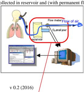
2. **Detailed scheme of interconnection of all setup components**. In all cases, connectors are designed so that they fit in suitable sockets only. O2 sensor, barometer and thermometer can be connected into any of 4 analogue ports (so not only as shown on the picture)
